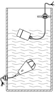
To ensure correct operation, the floating switches must be fixed (generally by their cables). The fixing mode depends on the switch type and is also described in the supplied product documentation.
