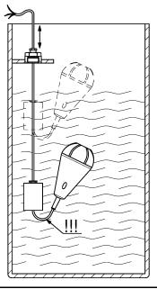
Here an example of the installation of a floating switch <u>SI/SSX/LF/4/1/K/PURLF/Variante</u>. with antistatic cable (with external conductive sheath) using the metallic fixing weight without potential equalisation terminal of the type
