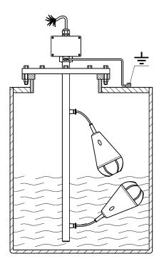
The immersion probe has to be included to the potential equalisation concept of the whole installation.
