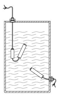
To mount a floating switch from the side using a stuffing gland, a <u>sleeve of</u> <u>corresponding size</u> must be present in the tank at the working height. You should position the sleeve in <u>line with the diagram " Switching action</u> in liquids with a specific gravity of 1g/cm<sup>3</sup> " in the supplied product documentation.
