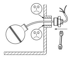
When mounting the floating switches, take care to ensure that the switch and in particular the cable are not damaged <u>by sharp edges and</u> <u>objects</u>.
