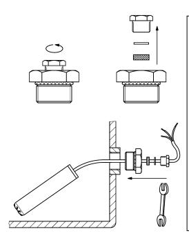
The **pressure screw should be tightened firmly but not so firmly** that it damages the gasket and the cable.
