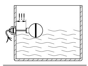
It is essential to ensure that the cable between the fastening point of the stuffing gland and the floating switch possesses at least the minimum length specified in the product documentation. If the cable does not possess at least the minimum specified length, this can lead to premature breaking of the wires and may also impair the
