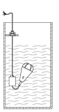
Only the fixing weight for antistatic cable, type <u>FG 55x93/Ex/KLF or FG 55x93/E/KLF/Ex</u> can be used for a
