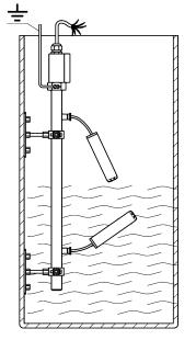
The immersion probe has to be included in the potential equalisation concept of the whole installation.
