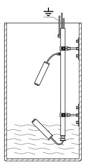
The metallic mounting pipe has to be included to the potential equalisation concept of the whole installation.
