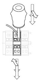
Push a screwdriver into the opening as shown in the drawing. Open the relevant terminal by pushing the screwdriver down towards the centre of the terminal block using a lever action.
