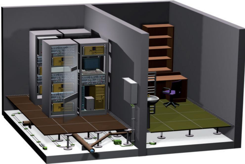
Monitoring of a false floor in a server room for the presence of an electrically conductive liquid using a cable electrode as well as a plate electrode in the adjacent room
