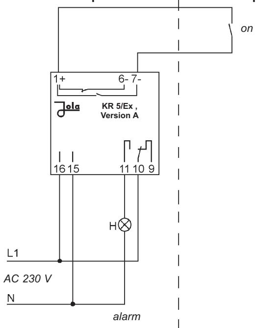
Non potentially explosive atmosphere | Potentially explosive atmosphere
