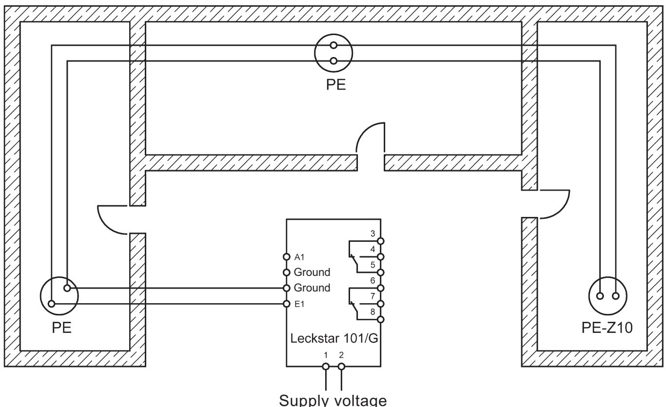
**Connection of several plate electrodes to one Leckstar 101/G electrode relay – group alarm**
