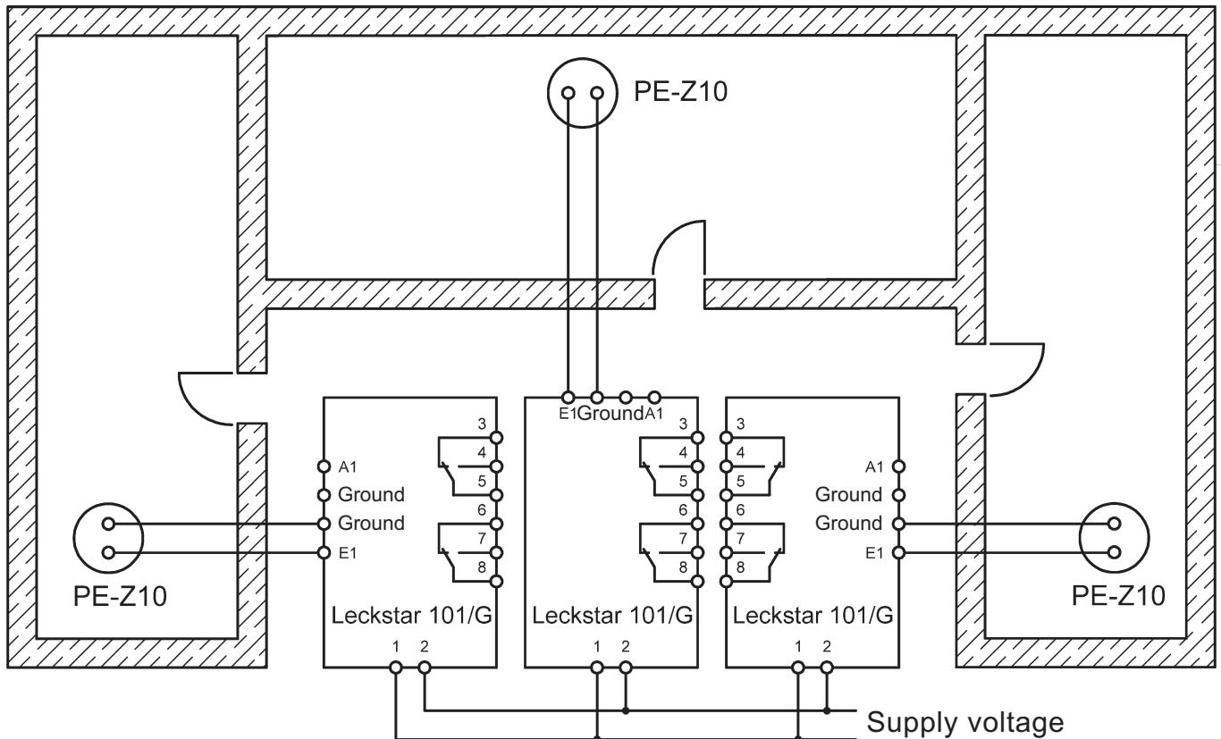
**Connection of several plate electrodes to several Leckstar 101/G electrode relay – separate alarm**
